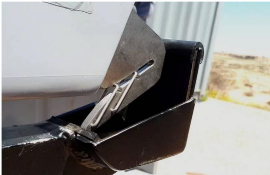
A close-up of the titanium rope capture 'carabiner' on the Insitu Integrator's wingtip. This grabs the rope when the UAV is commanded to fly home
