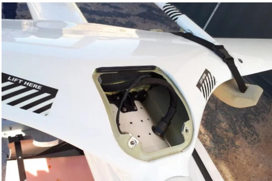
The interior of the Scaneagle 3 centre section. Note the multiple positions for the attaching bolts
