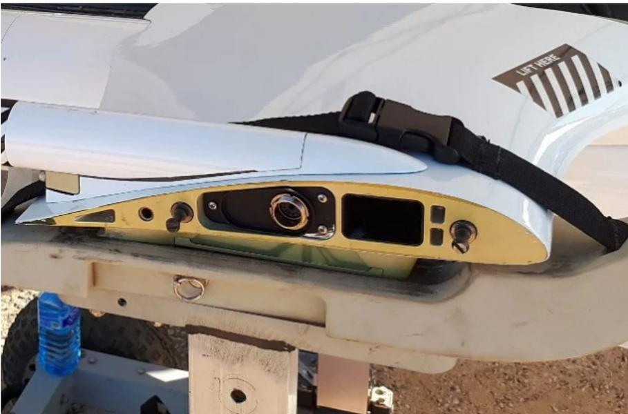
Insitu Scaneagle 3 wing root. Note the connectors for flap and aileron command cables. The main spar (not shown here) is carbon fibre
